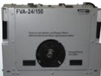
MAG direct current generator for charging aircraft batteries.
