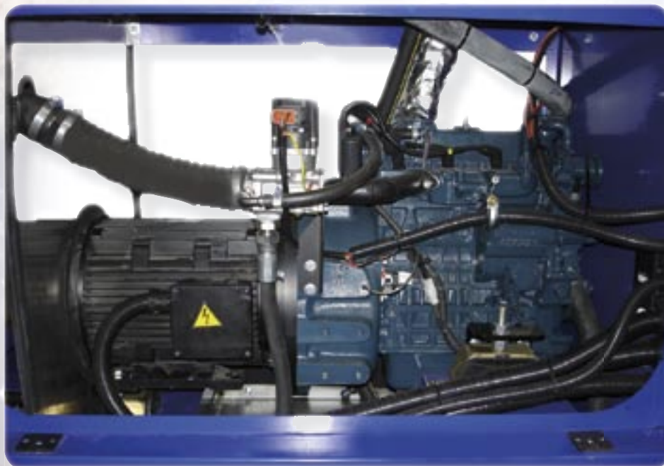
Symbol power generator with natural gas engine
